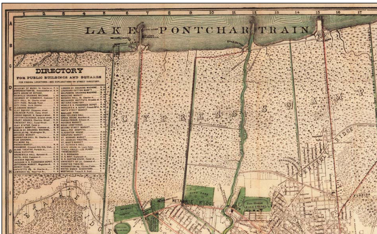
Figure 4.17: All 36 miles of drainage canals in the Lakeview and Gentilly areas are shown in this portion the 1878 Hardee Map (courtesy of The Historic New Orleans Collection). The canals are, from left: 17 th Street, New Basin (infilled), Orleans, Bayou St. John, and London Avenue, and the Lower Line Protection Levee.
