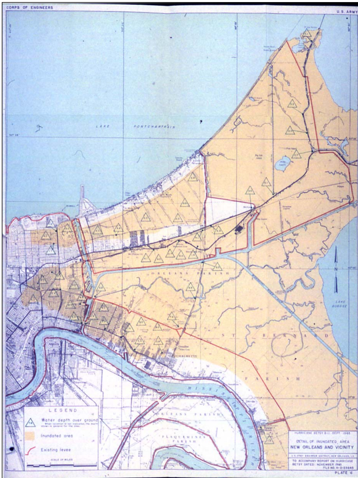
Figure 4.12: Portion of the flood inundation map from Hurricane Betsy in 1965, showing the areas on either side of the Inner Harbor Navigation Channel which were affected by overtopping, from storm surges on Lakes Borgne and Pontchartrain (from USACE, 1965).
