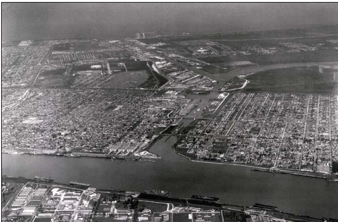
Figure 4.30: Aerial oblique view of the Inner Harbor Navigation Canal between 1960-64, after the entry to the Mississippi River-Gulf Outlet Channel had been enlarged (upper right), connecting to the inner harbor area (photo from the Army Corps of Engineers).
